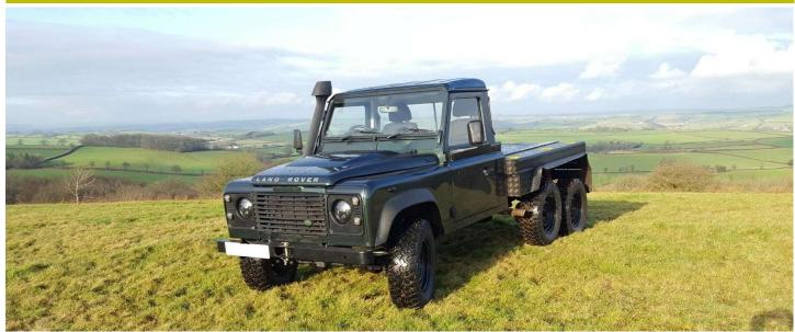
The Land Rover 6x6 HC Tandem Walking Beam suspension consists of a heavy duty tandem axle that can be installed on to a donor 110 or 130 chassis, converting the rear axle into a powered tandem axle walking beam suspension.
